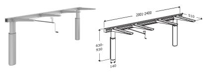
Manual lift for countertop. Lift for countertop, with a crank handle. Including 4 brackets. Lengths from 78.8"-94.5"/2001-2400 mm. Height adjustable 11.8"/300 mm.
