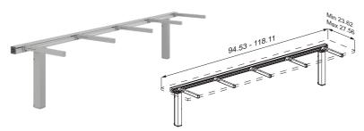
INDIVO lift for countertop, with two motors and control box. Max. load: 220 lbs/100 kg including the countertop. Incl. cross brace and five brackets.
