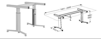
Manual lift for freestanding countertop. For countertops from 55.1" - 78.7"/1400 - 2000 mm. Height adjustable 11.8"/300 mm. Including 2 telescopic legs, longitudinal and cross braces and crank handle.
