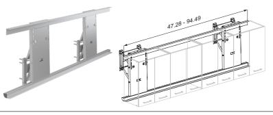
INDIVO lift for wall cupboards, with two motors and control box. Max. load: 485 lbs/220 kg including the cabinets. Height adjustable 16.9"/430 mm with switches or wired remote control. When height adjusting downward, the lift will also move 7.1"/180 mm towards the user. For wall cabinets width 47.3"-94.5"/1201-2400 mm.
